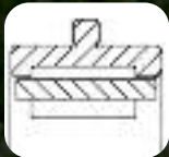
Flanged duplex ball bearing suitable for taking axial load in either direction. Axial clearance/preload to customers requirements.
