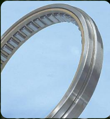
Roller bearing with flange in middle of outer race diameter, with locating slot and one piece bronze cage.
