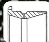
Flanged double row angular contact ball bearing with phenolic cage. Able to take axial load in either direction as well as radial load. Clearance/preload as required.
