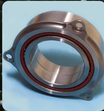
Flanged double row angular contact ball bearing with phenolic cage. Able to take axial load in either direction as well as radial load. Clearance/preload as required.
